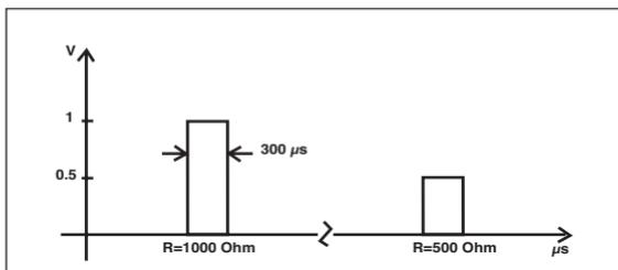
The maximum supplied current is the function of the resistance and of the duration selected, as shown in the following figure:
