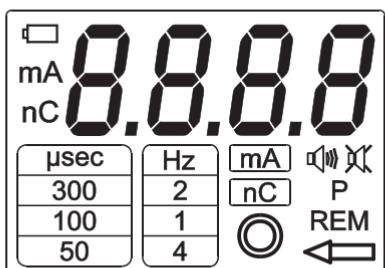
The display is used either for the visualization of the current or charge associated to each impulse, and for showing the selected parameters of functioning (duration of the impulse, frequency, measure unit of the visualization, active selector, and eventual battery alarm).
