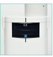
Set the desired aperture by selecting the appropriate aperture via the top rotating wheel on the prism body.
