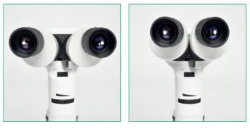
Set the required magnification by moving the magnification lever to the left (16x) or right (10x).
