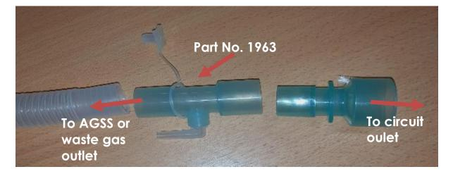
Step 2, push the larger wide silicone tube (ST08050) onto the side port
